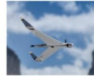
Orbiter 2b Aeronautics ca. 10 kg ca. 3 / 1.5 m / 0.4 m 33 – 50 kts (60-90 km/hm)
